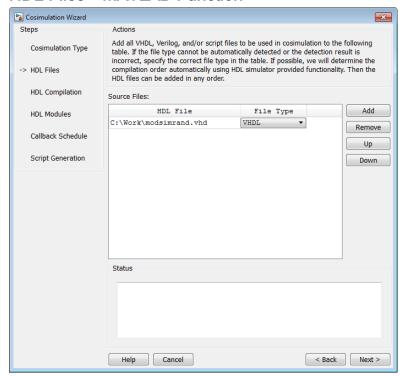
In the HDL Files pane, specify the files to be used in creating the function or block.
