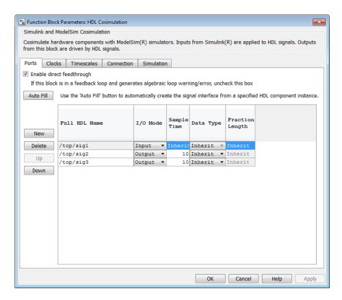
In this pane, you define the HDL signals of your design that you want to include in your Simulink block and set a sample time and data type for output ports. The parameters that you should specify on the **Ports** pane depend on the type of device the block is modeling as follows:
