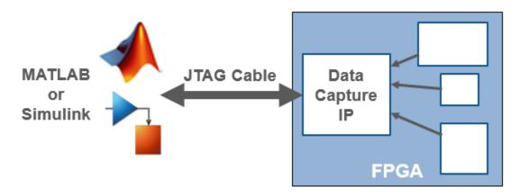
There are three major workflow steps to capture data from your FPGA board into MATLAB or Simulink. HDL Verifier provides tools to configure and execute the first and third steps. In between, you must manually integrate the generated IP into your FPGA design.
