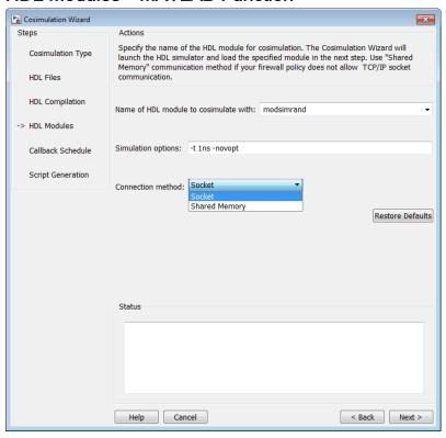
In the **HDL Module** pane, provide the name of the HDL module to be used in cosimulation.
