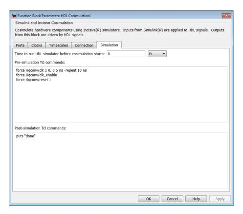
The following is an example of entering force commands in the **Simulation** pane of the HDL Cosimulation block for use with ModelSim:
