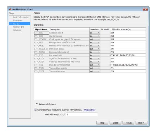
**Signal List**: Provide all the FPGA pin numbers for the specified signals. You can find this information in the board specification file. For vector signals, list all pin numbers on the same line, separated by commas.
