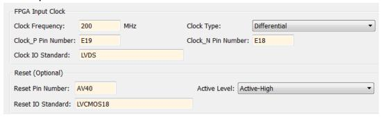
1 **FPGA Input Clock** — Clock details are required for both workflows. You can find all necessary information in the board specification file.
