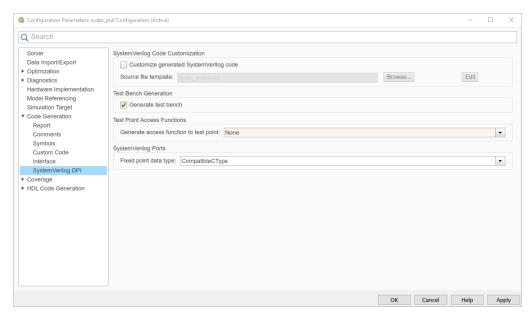
3 Click **OK** to accept these settings and to close the Configuration Parameters dialog box. Go to "Step 5. Generate SystemVerilog DPI-C Component" on page 30-4.
