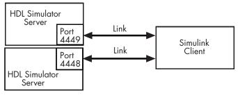
When you link the HDL simulator with a Simulink application, the simulator functions as the server. Using the HDL Verifier communications interface, an HDL Cosimulation block cosimulates a hardware component by applying input signals to and reading output signals from an HDL model under simulation in the HDL simulator.
