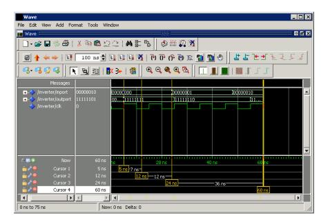
Now consider a cosimulation of the same model, this time configured with a scale factor of 100 in the **Timescales** pane.
