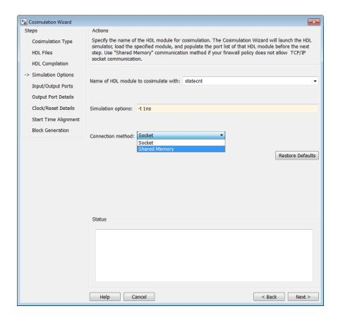
In the **HDL Modules** pane, provide the name of the HDL module to be used in cosimulation.
