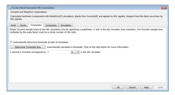
When you click **Determine Timescale Now**, HDL Verifier connects Simulink with the HDL simulator so that it can use the HDL simulator resolution to calculate the best timescale. You can accept the timescale HDL Verifier suggests or you can make changes in the port list directly. If you want to revert to the originally calculated settings, click **Use Suggested Timescale**. If you want to view sample times for all ports in the HDL design, select **Show all ports and clocks**.
