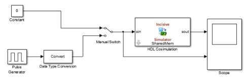
The model contains an HDL Cosimulation block (labeled HDL\_Cosimulation1) simulating an 8-bit inverter that is enabled by an explicit clock. The inverter has a single input and a single output. The following code excerpt lists the Verilog code for the inverter:
