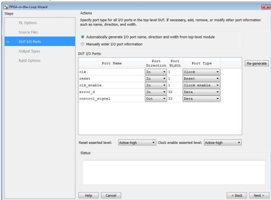
Step 5: Verify DUT I/O Ports for FIL Block
