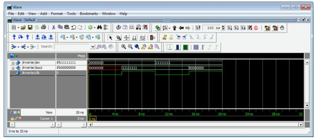
5 In the Simulink model, change **Constant value** to 2 and **Sample time** to 20 and start another simulation. This time, the value in the Display block changes to 253 and the ModelSim **wave** window appears as shown in the following figure.
