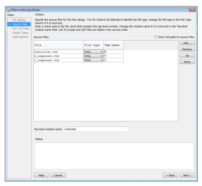
The FIL Wizard automatically fills the **Top-level module name** field with the name of the selected HDL file; in this case, **Controller**. In this example, the top-level module name matches the file name so that you do not need to change it. If the top-level module
