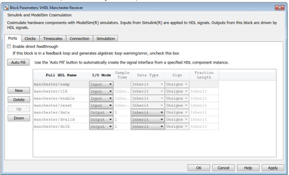
**Note** When you define an input port, make sure that only one source is set up to force input to that port. If multiple sources drive a signal, your Simulink model may produce unpredictable results.
