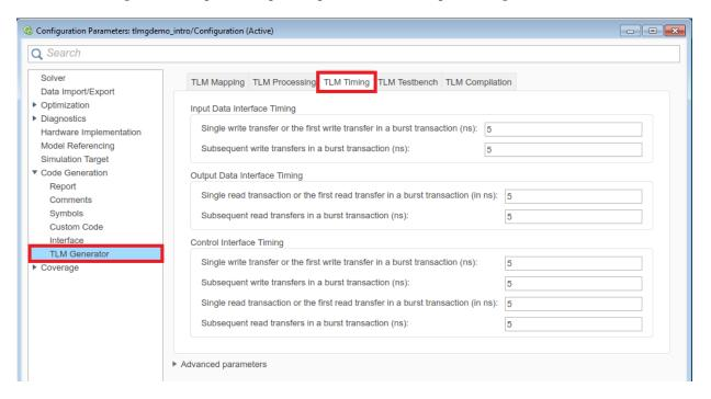
For this example, the input and output delays are counted with wait() in the interface or, if the temporal decoupling is enabled, they are annotated to the received transaction and sent back to the initiator. Set a time value of 5ns for each of the transactions of **Input Data Interface Timing**, **Output Data Interfacing Timing**, and **Control Interface Timing**.
