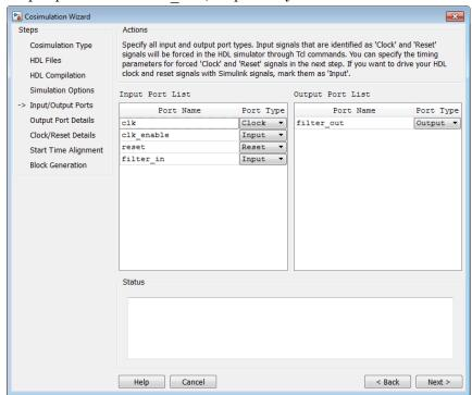
The Cosimulation Wizard attempts to identify the port type for each port. If the wizard incorrectly identifies a port, you can change the port type using these tables.
