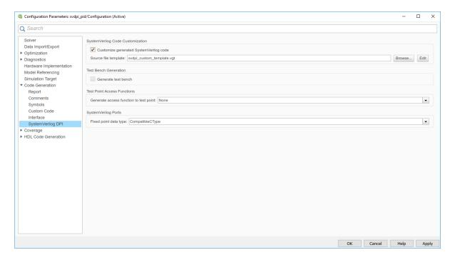
You can select **Edit** to see the contents of the template. The following example shows the content of the template file provided with HDL Verifier,
