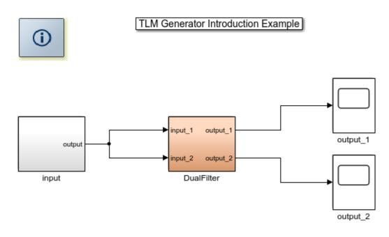
This model shows the TLM component generation with a dual 4 taps FIR filter.
