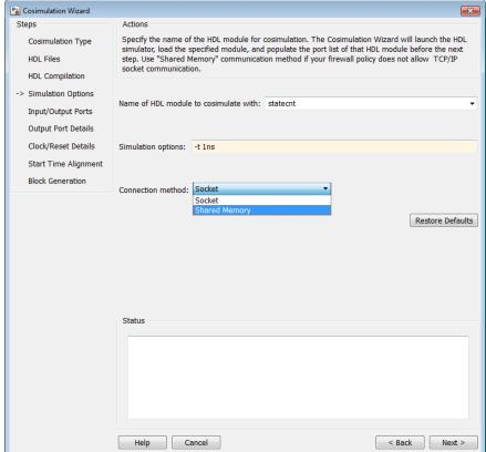
In the **Simulation Options** pane, provide the name of the HDL module to be used in cosimulation.
