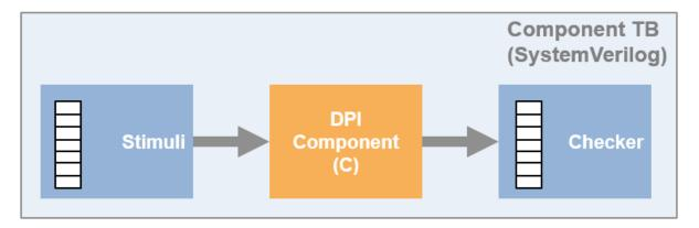
If you enable logging on test points in your model, the generated test bench also compares their signal values in the SystemVerilog component with logged values from Simulink.
