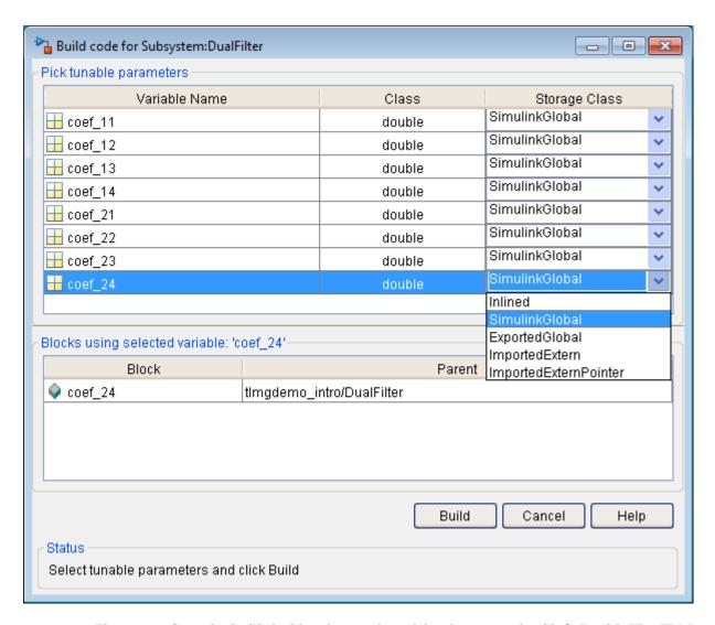
The option **Simulink Global** has been selected for this example. Click **Build**. The TLM generation is completed when you see the following message appear in the MATLAB command window:
