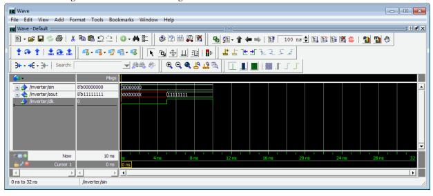
4 In the Simulink model, change **Constant value** to 255, save the model, and start another simulation. The value in the Display block changes to 0 and the ModelSim **wave** window is updated as follows.
