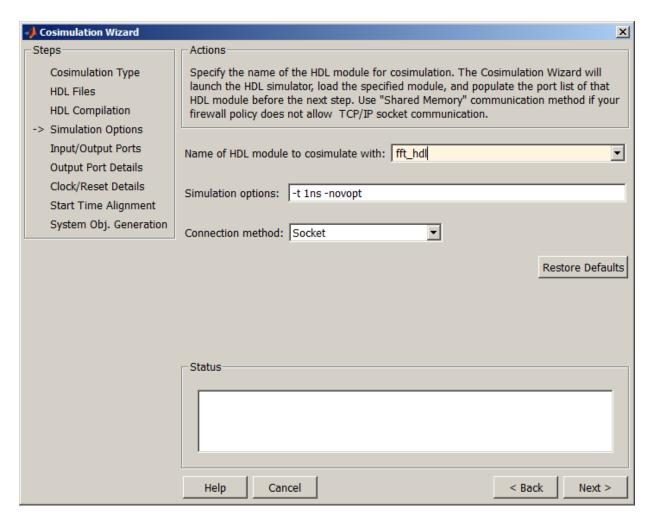
**c.** Click **Next**. The Cosimulation Wizard launches the HDL simulator in the background console using the specified HDL module and simulation options. If the wizard launches the HDL simulator successfully, the wizard populates the input and output ports on the Verilog model **fft\_hdl** and displays them in the next step.
