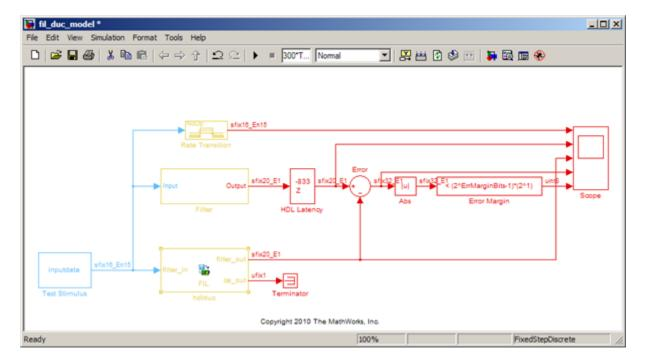
Run simulation. Observe the output waveforms from the behavioral filter block, the FIL block, and the error margin. Because the behavioral filter block does not have pipeline registers, there are small differences between the behavioral filter block output and the FIL block output. These errors are within the error margin.
