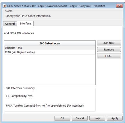
The Interface page describes the supported FPGA I/O Interfaces. Select any listed interface and click **View** to see the **Signal List**. If the board definition file has write permission, you can also **Add New** interface, **Edit** the interface, or **Remove** an interface.
