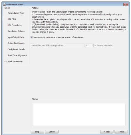
1 Specify if you want HDL Verifier to determine the timescale when you start the simulation by selecting **Automatically determine timescale at start of simulation**. If you prefer to determine the timescale yourself, leave this box unchecked and enter the timescale value in the text boxes below. The default is to automatically determine timescale.
