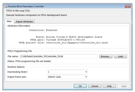
3 A message window indicates when the FPGA programming file has loaded as expected. Click **OK**.
