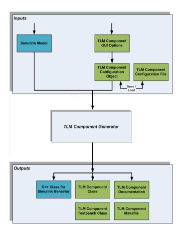
After code generation is complete, you can then use these generated files (outputs) to create the standalone TLM executable. See "Export TLM Component" on page 25-2.
