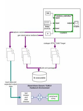
The following general workflow describes the process for creating an OCSI-compatible TLM component representing the Simulink algorithm:
