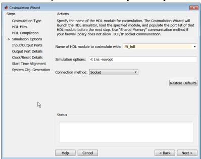
In the **HDL Module** pane, provide the name of the HDL module to be used in cosimulation.
