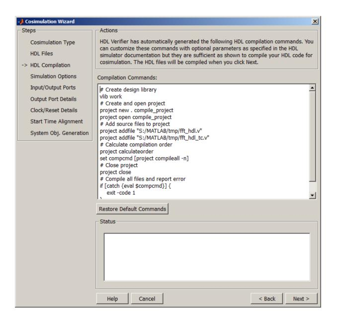
Click **Next**. The MATLAB console displays the compilation log. If an error occurs during compilation, that error appears in the Status area. Correct the error before proceeding to the next step.
