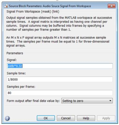
The sample rate and frame size of the input signal propagate throughout the model.
