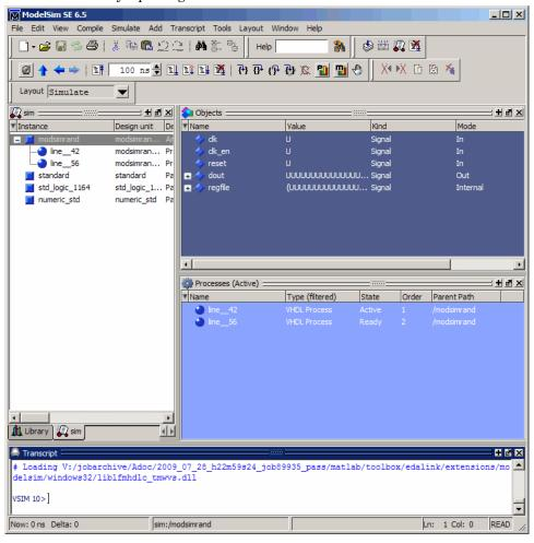
2 Initialize the simulator for verifying modsimrand with MATLAB. You initialize ModelSim by using the HDL Verifier matlabtb command. This command defines the communication link and a callback to a MATLAB function that executes in MATLAB on behalf of ModelSim. In addition, the matlabtb command can specify parameters that control when the MATLAB function executes.
