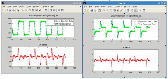
This difference occurs because the Simulink signal capture necessarily makes the signals discrete and thus the same exact data is not used in both the Simulink and stand-alone SystemC simulations. You can improve the fidelity of the discrete signal simulation in SystemC by choosing a smaller fundamental step size in Simulink before clicking **Verify TLM Component**.
